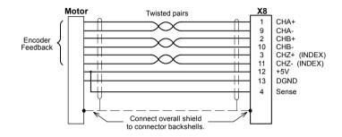
Figure 13 - Encoder cable connections without halls - rotary motors
