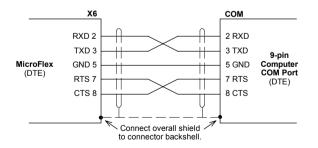
Figure 35 - RS232 serial port connections
