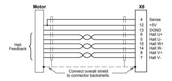
Figure 14 - Halls-only feedback cable connections - rotary motors
