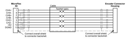
Figure 52 - Encoder signal cable grounding
