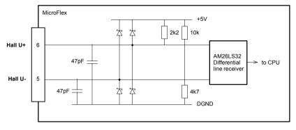
Figure 11 - Hall channel input circuit - U phase shown
