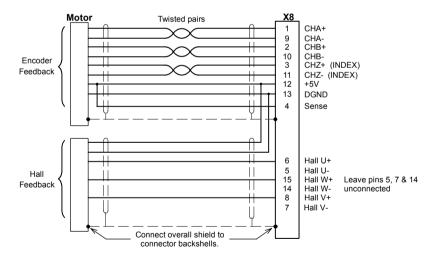
Figure 15 - Encoder cable connections - linear motors
