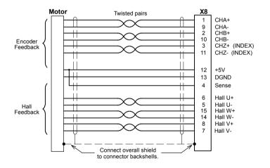
Figure 12 - Encoder cable connections - rotary motors
