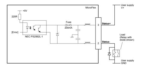
Figure 33 - Drive status output circuit
