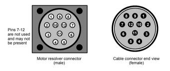
Figure 19 - Baldor motor resolver cable pin configuration
