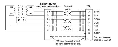
Figure 18 - Resolver cable connections
