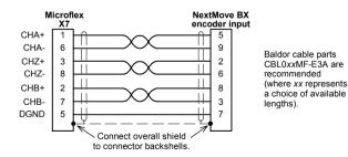
Figure 22 - MicroFlex encoder output to NextMove BX encoder input
