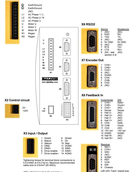
(NC) = Not Connected. Do not make a connection to this pin.
