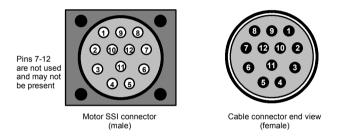
Figure 17 - Baldor motor SSI feedback cable pin configuration
