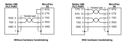
Figure 37 - RS232 cable wiring
