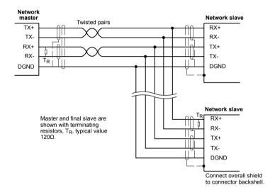
Figure 36 - 4-wire RS422 multi-drop connections
