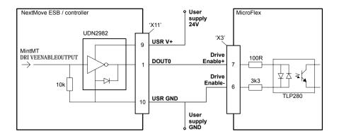
Figure 28 - Drive enable input - typical connection from a Baldor NextMove ESB
