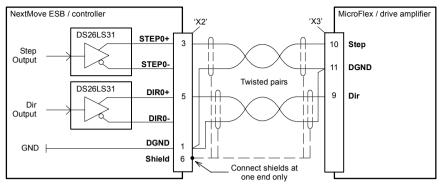
Figure 32 - Stepper input - typical connection from a Baldor NextMove ESB
