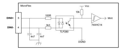
Figure 29 - General purpose digital input circuit
