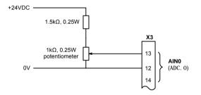
Figure 25 - Typical input circuit to provide 0-10V (approx.) input from a 24V source
