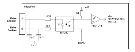
Figure 27 - Drive enable input circuit
