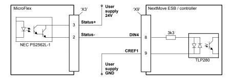
Figure 34 - Status output - typical connections to a Baldor NextMove ESB
