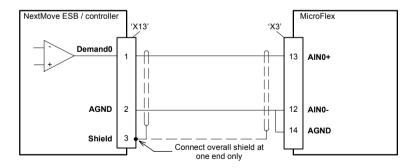
Figure 26 - Analog input - typical connection from a Baldor NextMove ESB
