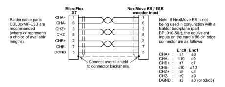
Figure 21 - MicroFlex encoder output to NextMove ES / ESB encoder input
