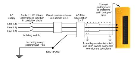
Figure 3 - Single or three-phase power connections
