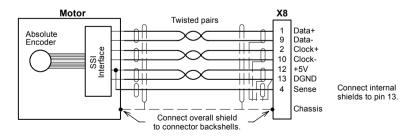
Figure 16 - SSI encoder cable connections
