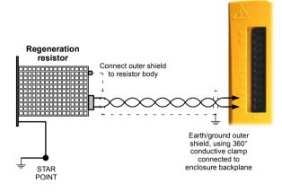
Figure 9 - Regeneration resistor connections
