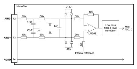
Figure 23 - AIN0 analog input (demand) circuit
