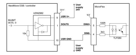
Figure 30 - Digital input - typical connection from a Baldor NextMove ESB
