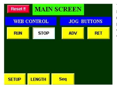
This is the Main Screen with a Reset button. This feature will remain On(even if you cycle the power), until the Reset code is entered once more (see above)
