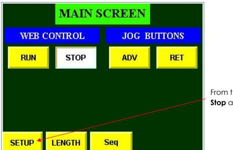
From the main screen **Press Stop** and then **Press SETUP**
