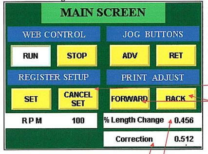
After the first mark arrives the Normal Register Screen Appears. The Jog buttons no longer move the print.
