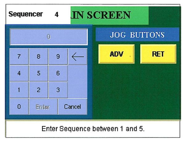
The Sequence is used to make the Register system follow the same pattern as the original print cylinder. For example if two repeat patterns were printed per rotation of the Print Cylinder a sequence of two will cause the controller to look at every second mark, thereby following the original print cylinder pattern. The controller may be programmed to look at every mark Seq. = 1, every second mark Seq. = 2, every third mark Seq. = 3, every fourth mark Seq. = 4, or every fifth mark Seq. = 5,
