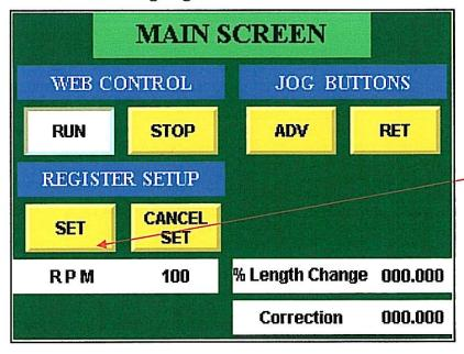
At this point the Set button has been pushed and the controller is waiting to see the first register mark. The Set button will blink On and Off until a mark is seen.
