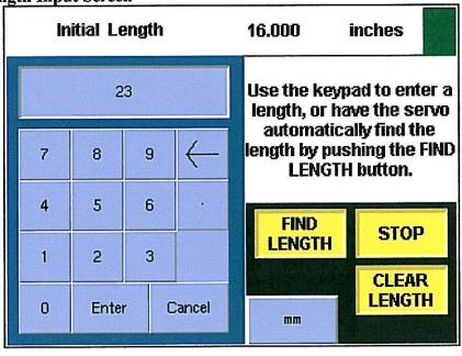
There are two methods to input the length. One is to Enter the Length directly in inches or millimeters.
