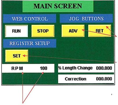
The Screen is in Run Mode. Begin running the machine, the draw rollers will feed the correct amount of web based on the previously entered length.
