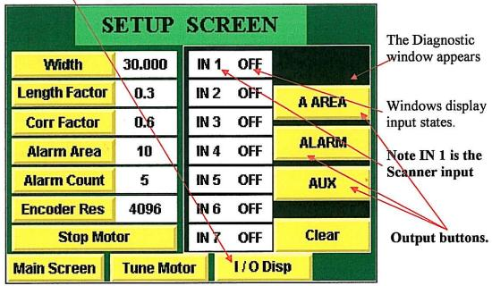
The states of the inputs are shown in the I/O screen above. IN 1 is always used to show the scanner state. If the output led on the scanner is on then the pickup LED should turn on and the IN 1 display above should change to "ON".
